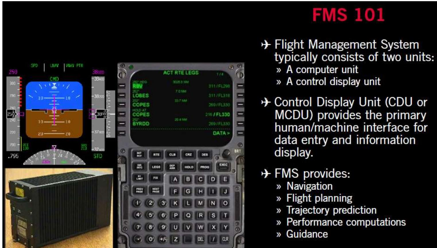
The image displays a Flight Management System (FMS) interface and hardware. On the left, a cockpit display shows various parameters: SPD (259), LNAV, VNAV, PTH, and a central CMD display. Below this is a physical FMS unit. On the right, a Control Display Unit (CDU) shows the 'ACT RTE LEGS' screen with the following data:
